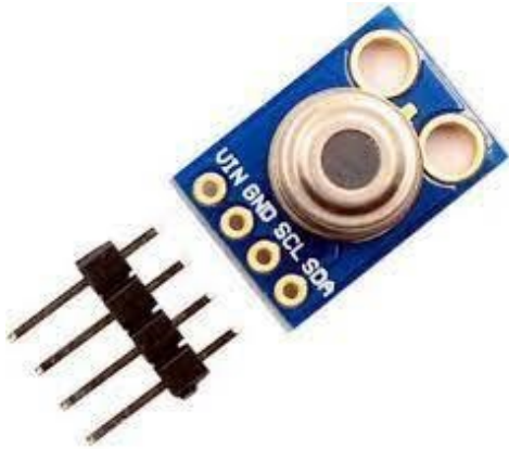
Figure 3: Image of a Temperature sensor MLX90614 src:- Circuit digest
